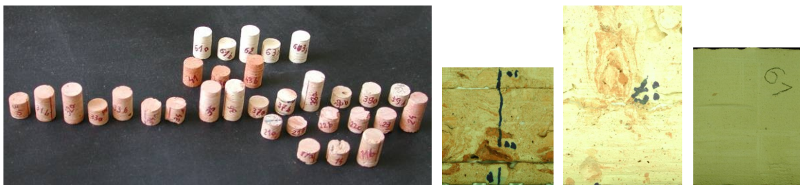
Figure 3: Set of micro-core specimens and unwrapped surfaces of micro-cores No 22, 37, 61 from layers 5, 6 and 14 respectively
